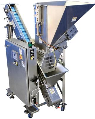
metered continuous flow of bulk products like cooked pastas and rice, cut vegetables, fruits, meats, and various salads to the hopper of its volumetric cup filler, allowing large quantities to be placed into the hopper with minimal monitoring.
