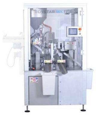
Oystar Group's tube filling platform is highly productive and ergonomically designed for maximum process reliability through servo technology and excellent accessibility from all sides.
