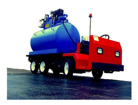
CECOR introduces the extra power combination coolant sumpcleaner/dispenser, Model CP50-200/200CB5, for coolant recycling programs in larger metal machining operations. Tank consists of two compartments; one 200-gallon for collecting and filtering dirty coolant and another 200-gallon for dispensing clean coolant.
