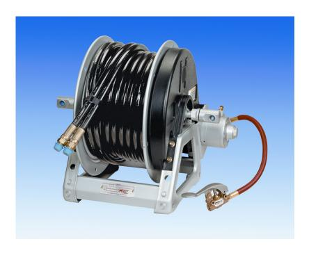
Ideal for hydraulics, air/water and spray painting applications, 2000 Series reels from Hannay Reels are built to handle pressures up to 3000 psi (207 bar) and temperatures from 20 to 400 degrees Fahrenheit (minus-seven to 204 degrees Celsius).
