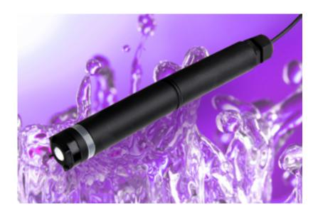
Sensorex's FCL500 series free chlorine sensors use advanced amperometric measurement technology to provide highly accurate monitoring of free chlorine in process applications. With three models covering the 0-2ppm, 0-5ppm and 0-10ppm ranges, FCL500 sensors can be used in new installations or as a field replacement for existing sensors.
