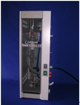
The new LabStrong Fi-Streem 2S Stills from LabStrong Corporation and Fi-Streem International produce four liters of product water per hour and are available in two models, A74420LS and A74428LS. The stills consistently produce high quality ASTM Type II water and remove inorganic ions, dissolved gasses, organics, particles, bacteria, pyrogens and nucleases from water.
