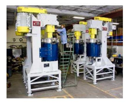
Union Process has unveiled its QL-100 Circulation Attritors with the capability to take high pumping rates that result in a faster grind and a narrower particle size distribution. According to the company, these high-production grinding mills additionally grant:
