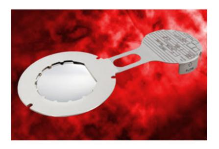
According to Oseco, its PRO+KRGL reverse buckling rupture disc provides a best-in-class Kr value (which is used to determine the frictional flow loss through a rupture disc and holder) for improved flow, which permits the use of smaller piping. The company says that the disc further grants:
