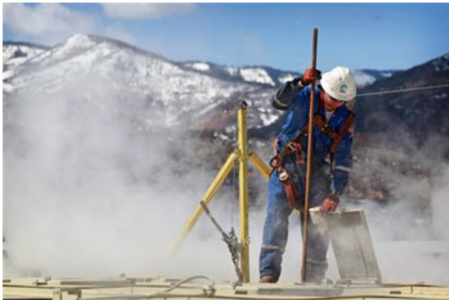
In this March 29, 2013 photo, a worker checks a dipstick to check water levels and temperatures in a series of tanks at an Encana Oil & Gas (USA) Inc. hydraulic fracturing operation at a gas drilling site outside Rifle, Colorado. Hydraulic fracturing, or "fracking," can greatly increase the productivity of an oil or gas well by splitting open rock with water, fine sand and lubricants pumped underground at high pressure. Companies typically need several million gallons of water to frack a single well. In western Colorado, Encana says it recycles over 85 percent of the water it uses for fracking to save money and limit use of local water supplies. (AP Photo/Brennan Linsley)
