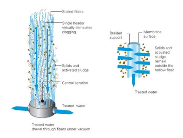
The free moving fibers, combined with central air scour aeration, ensure stable filtration during plant operation, long membrane life, and lower operating costs due to reduced need for energy, cleaning and maintenance.
