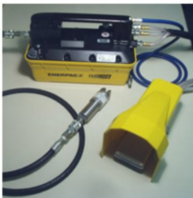
Scissor-style handset & jaws with hydraulic / pneumatic pump and remote footswitch.
