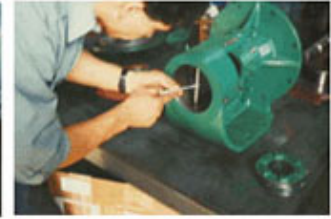
Check bearing housing for proper fit. Take various readings to make sure that the housing is not ovalized. Check for wear marks that would indicate that the outer race of the bearing has been spinning inside the housing. Bore size should be 5.514"/5.512"
