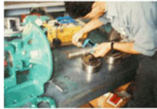
Check bearing journals for proper tolerance (in this case shaft should be 2.1650"/2.1645")
