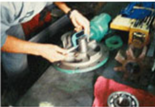
Check the head pin for proper tolerance and irregular wear. Diameter should be 2.5625"/2.5615"
