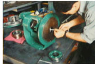
After pressing carbon bushing in bearing bracket, check I.D. of bushing for proper tolerance. It should be 2.4445"/2.4425"
