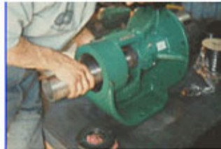
Pre-cut the necessary number of packing rings, lubricate each piece of packing with bearing grease and proceed to pack the first ring to the bottom of the stuffing box with the aid of a pipe. It is very important that each piece of packing be snugly pressed against the previous piece. If a pipe is not available use pack rods. DO NOT USE A SCREWDRIVER.
