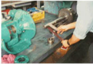
Clean and deburr shaft and rotor
