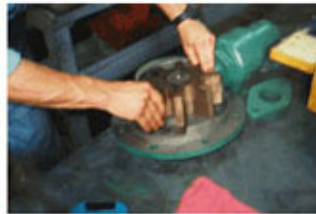
After pressing carbon bushing in idler, check I.D. of bushing for proper tolerance. It should be 2.5700"/2.5720" Place idler over head pin and rotate by hand to insure that there is no interference.
