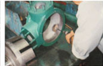
Clean and deburr the inside of the volute with the aid of a drill and an emery flapper.
