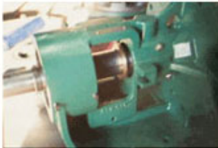
Lightly lubricate the inside of the carbon bushing. (bearing oil or grease is fine) Then install rotor in place and rotate same by hand to make sure that it spins free. Make sure that the packing retainer washer is in place.
