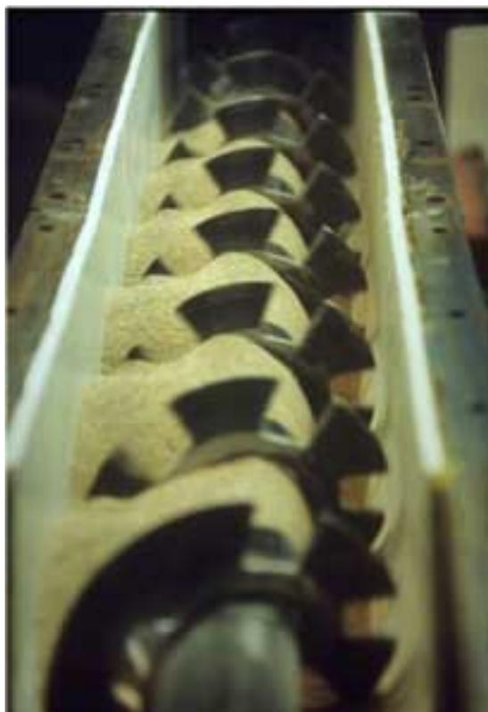
**Figure 1: Continuous blending screw interior**
