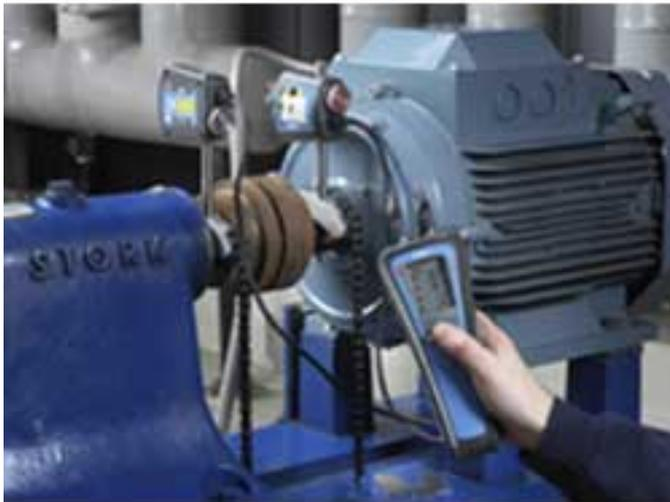
A growing number of food and beverage manufacturers are turning to advanced shaft and belt alignment systems, often equipped with laser sighting. The trend, which affects diverse food sectors, is fueled by the prospect of lower energy costs, reduced downtime and better overall machine reliability.
