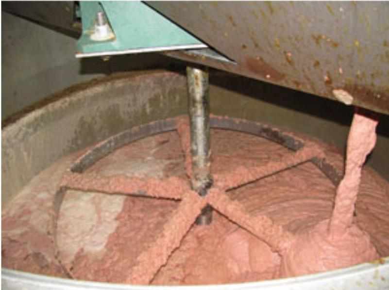
The original system at Chenango Valley Pet Foods (CVPF) consisted of a stainless steel tank on legs with a dual hose peristaltic pump with an inverter drive. The pump discharged through a 2-inch sanitary tube line and passed through a 1-inch Coriolis-style flowmeter on its way to the mill/extruder.
