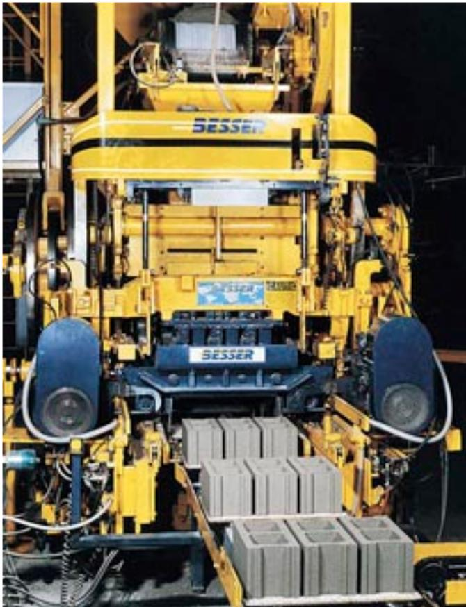
Each motor on the horizontal conveyor, the vertical elevator and the finger cars are equipped with MagnaShear oil shear brakes, on motors from  $\frac{3}{4}$  to 5 HP. The totally enclosed oil shear design dissipates heat and is impervious to dust and dirt.
