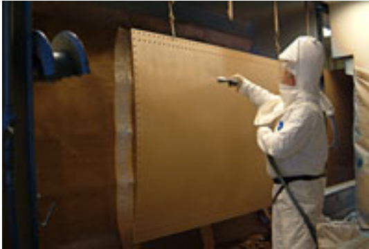
The key difference in coatings lies in the application process. The highest quality coatings are applied at the factory and cured in environmentally controlled circumstances.
