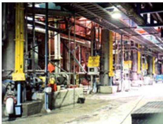
*Rod-type nuclear sources are mounted on standpipes.*
