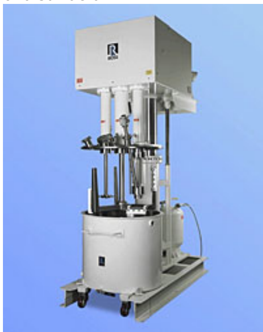
This 100-gallon VersaMix high-shear mixer is equipped with a SLIM induction tube for subsurface introduction of powders right into the high shear zone.
