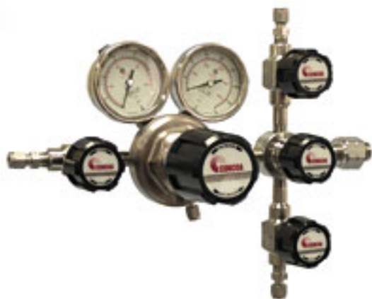
Figure 1: The 455 Series regulator features internal Hastelloy components and Monel gauges for improved corrosion resistance over 316L stainless steel
